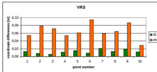
**Figure 2.** Position differences of control network points determined using VRS service
