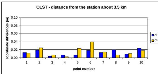
**Figure 4.** Position differences of control network points determined using OLST reference station
