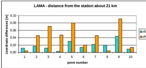
**Figure 3.** Position differences of control network points determined using LAMA reference station
