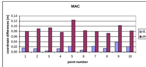
**Figure 1.** Position differences of control network points determined using MAC service
